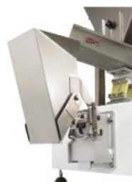
Stepper Motor operates the Weigh Bucket Gate
